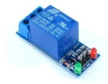
Gambar 2.3 Modul Relay 1 Channel
